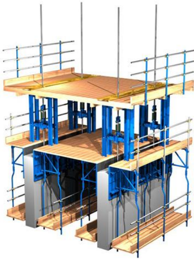
Basic Slipform Rig
