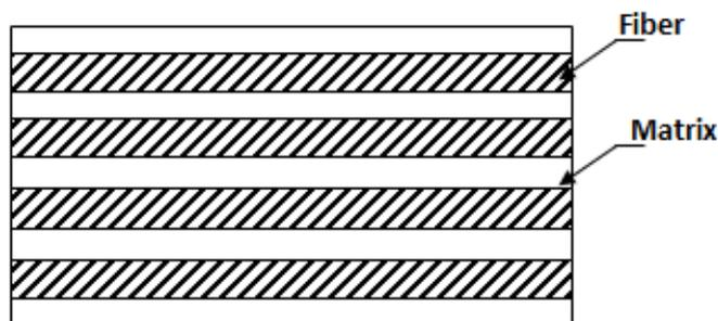
**Figure (2.1) Structure of a fibrous composite**
