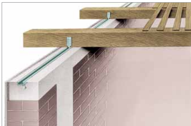
Typical installation of timber beams using HNA nailing straps with HALFEN Cast-in channels embedded in concrete.
