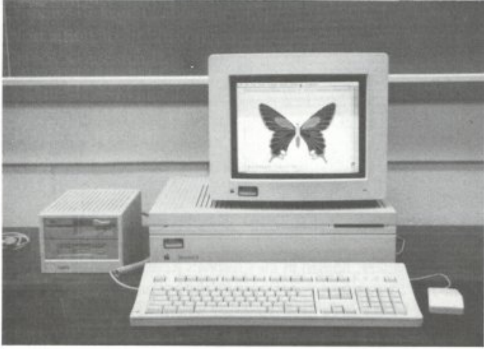
The DaynaFile is connected to a Macintosh II microcomputer and is available for use in the Graphics Research Laboratory, Room 114 Computer Center.
