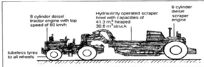
**Figure- typical 2 and 3 axial scraper**
