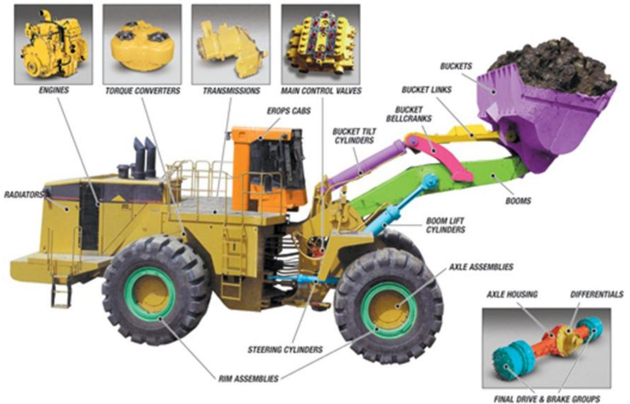
A shovel is also known as a front-end loader, loader, a bucket loader or sometimes a scoop loader. it is a bucket that is on the end of movable arms. it tilts and is used to lift and move material. the shovel is part of a tractor. it is either a permanent-mounted version or a removable attachment. the bucket at the end of the arms can be replaced with other tools, such as forks for lifting pallets or bale tools that are specifically designed to handle bales of hay.
