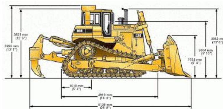
The blade is used to push, shear, cut, and roll material ahead of the tractor. The bulldozer is an effective and versatile earthmover. Bulldozers are used as both support and production machines on many construction projects.
