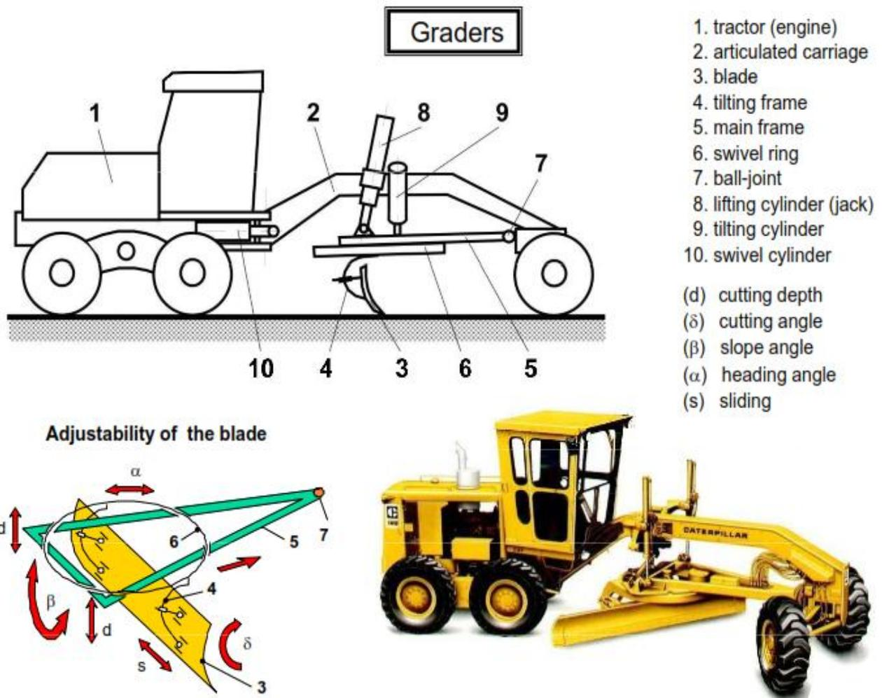
*Figure - Principal parts of a motor grader.*
