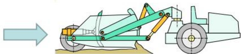
Discharging (spreading and compacting): apron up (open), bowl up, ejector forward
