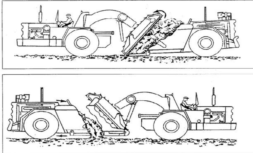
*Figure- Typical Elevating Scraper*
