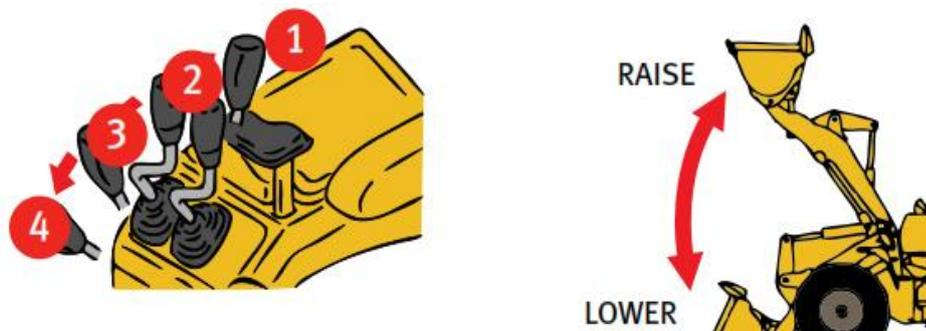
The controls to tip the bucket are: 1. Roll back, crowd or tilt 2. Hold 3. tip or dump
