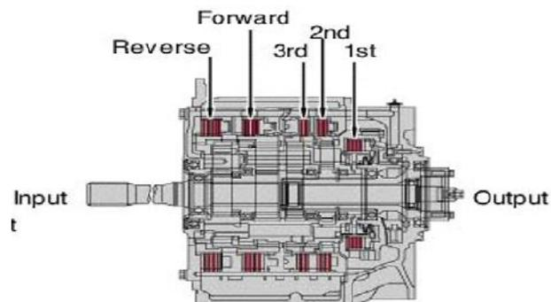
Planetary gear type transmission
