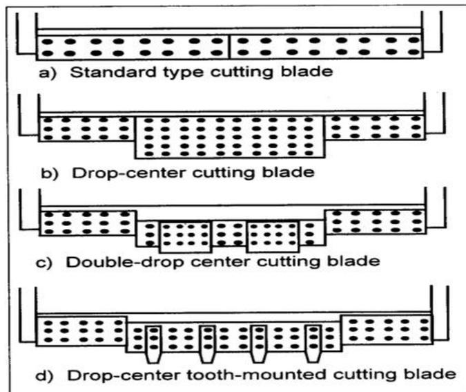
*Figure – Cutting blade for Scraper*
