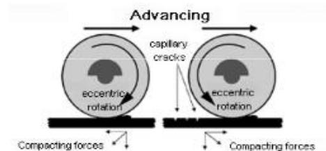
Effect of direction of rotation on the quality of compacted surface
