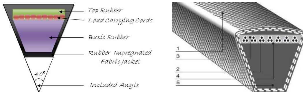
Figure 8-12: Cross section of V-Belt
