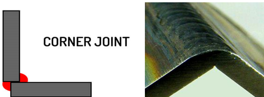
Figure 3-5: Corner joint welding
