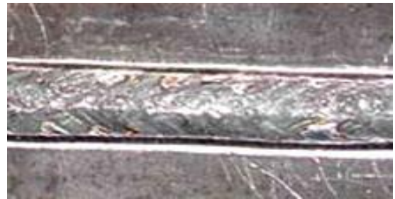
Figure 3-4: Butt joint welding
