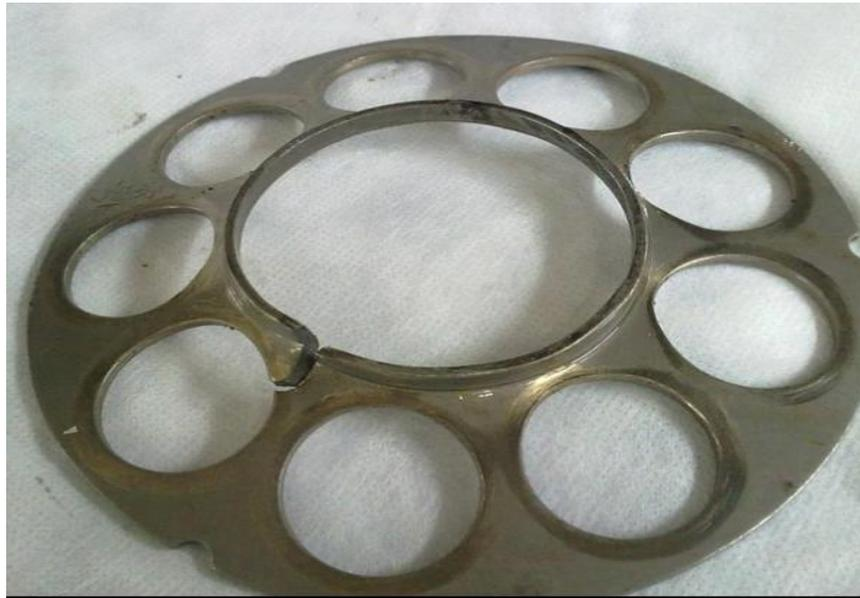
**Figure 3-26 motor plate damaged**
