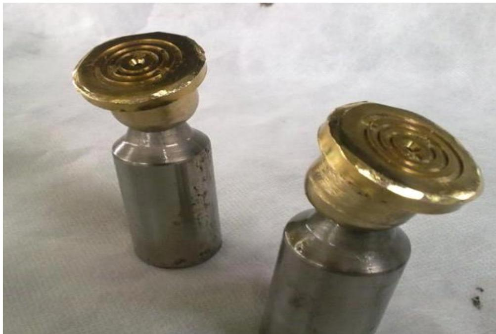
**Figure 3-25 motor pistons damaged**
