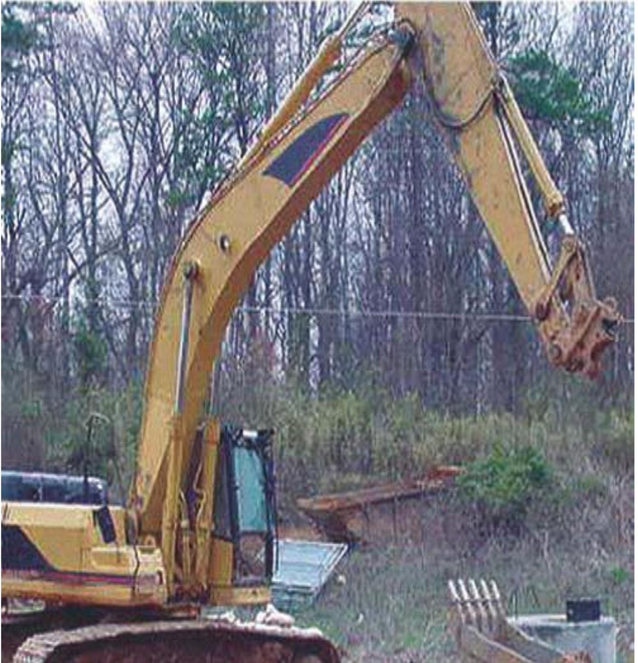
**Figure 4-3 excavator bucket damage and falling down**
