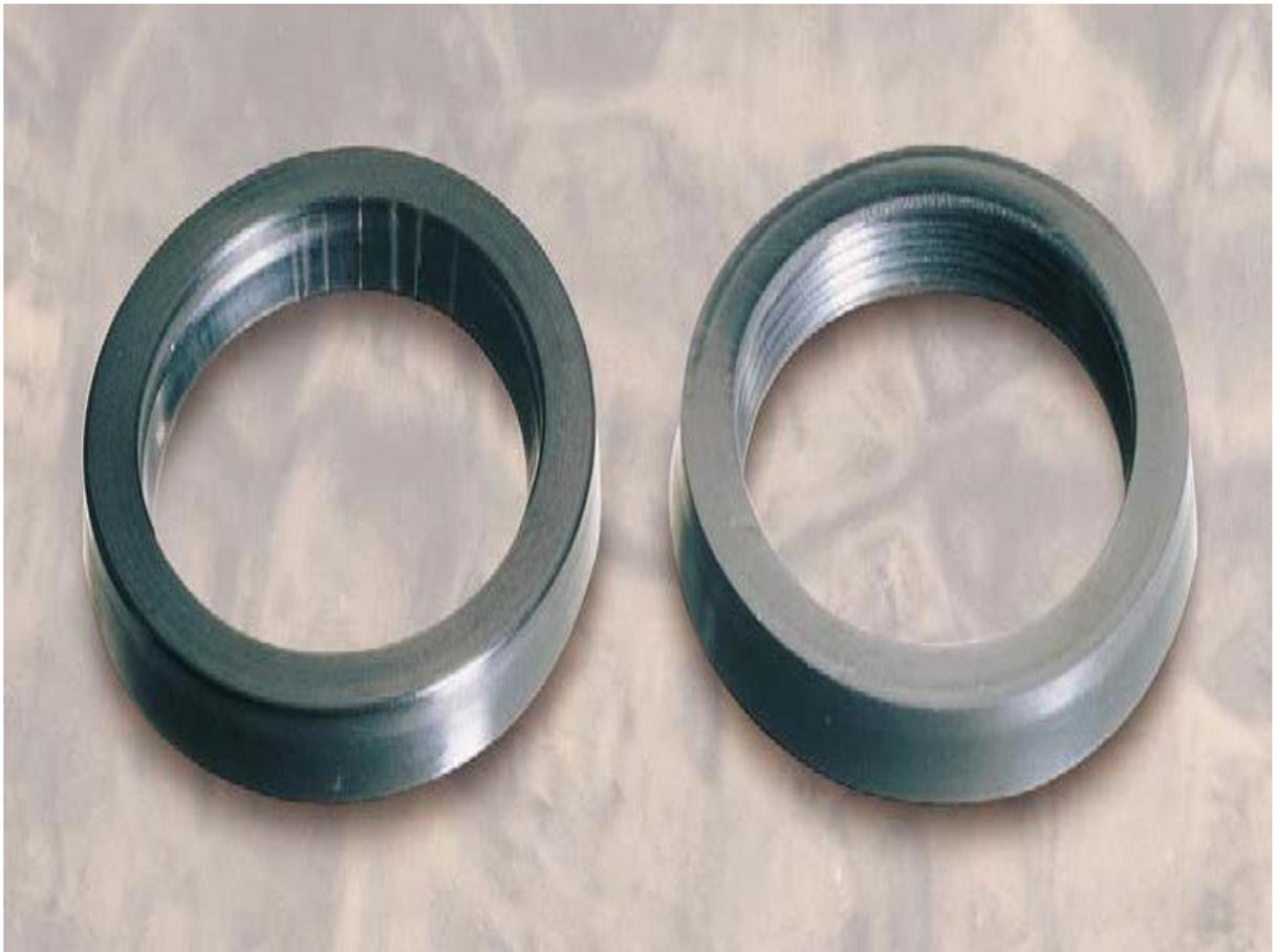
**Figure 2-29 Contamination damage is apparent in this rod seal, where the serrations are worn completely away. The seal on the right is a new one, shown for comparison.**
