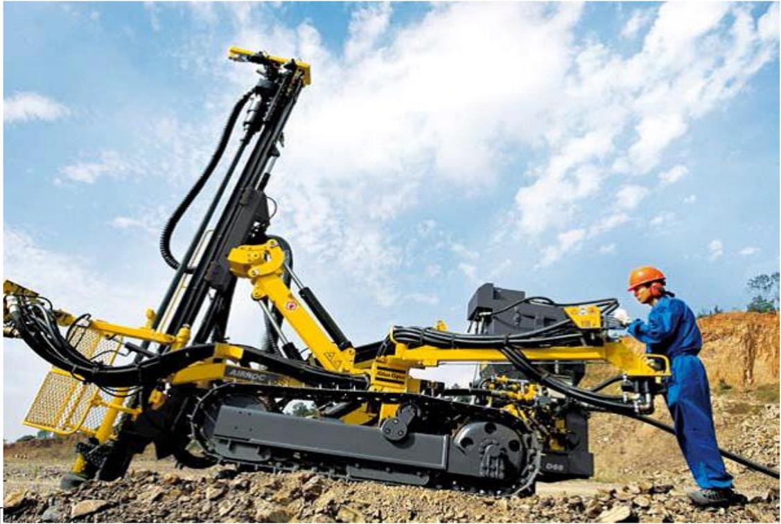
**Figure 3-30 another type of drilling machine which is used in surface mining**
