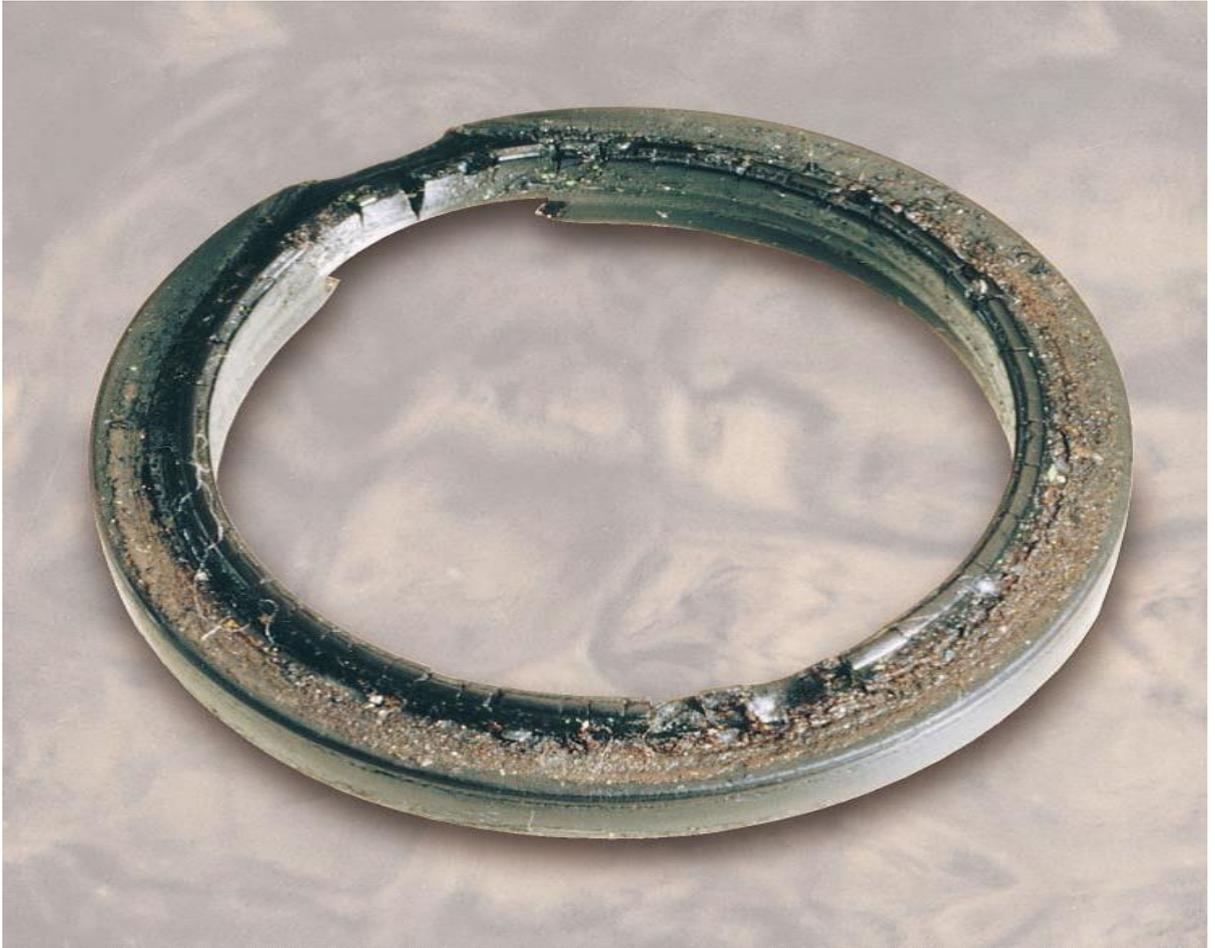
**Figure 2-32 wiper seal damage caused by excessive heat**
