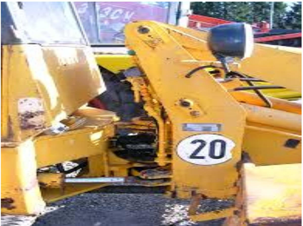
**Figure 3-6 wheel loader 966C - steering cylinder**
