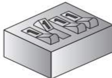
Rocker-type DIP switch
